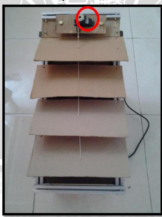
Penempatan *Continuous Rotation Servo Motor*
