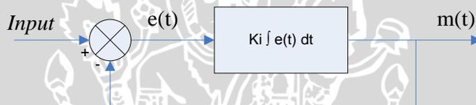
Gambar 2.8 Diagram Blok Kontroler Integral
