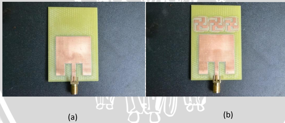
Figure 4.6 Front side of fabricated microstrip patch antenna ( a ) without EBG ( b ) with EBG.
