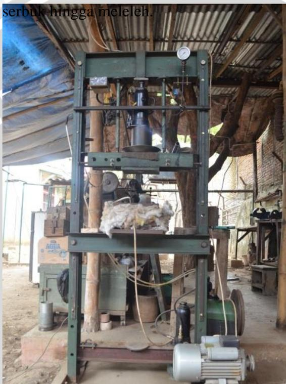
Gambar 3.1 Mesin *Hot Pressing*
