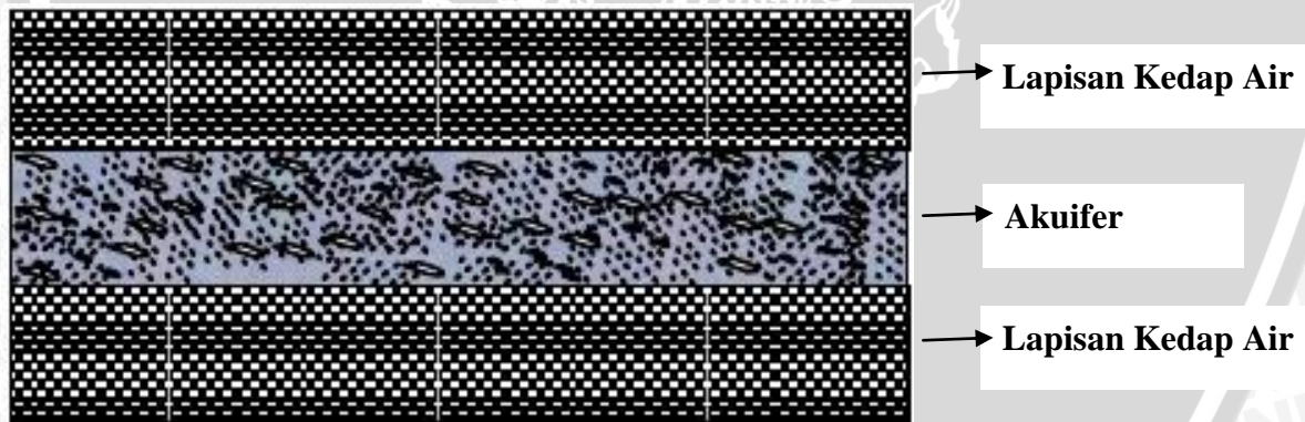
Gambar 2.4. Akuifer Tertekan ( Confined aquifer )
