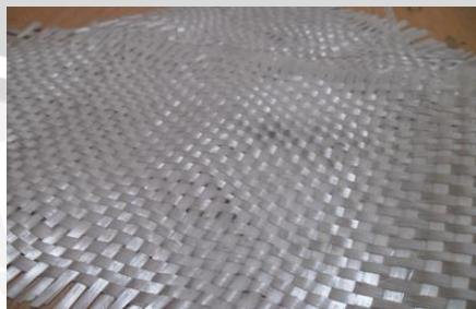
Gambar 3.12 Serat *fiber E-Glass woven roving*.
