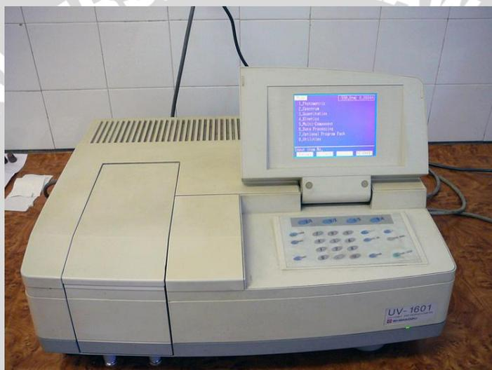
Gambar 2. 10. *Spectrophotometer UV-1601*
