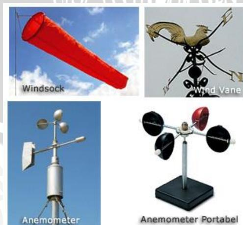
Gambar 2.2 Macam-macam Alat Pengukur Angin
