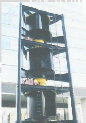
Gambar 2.2 tiga-stack savonius Sumber: Marnoto Tjukup (2010)
