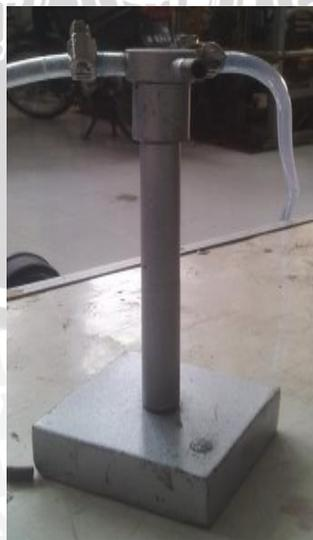
Gambar 3.4 Combustor holder
