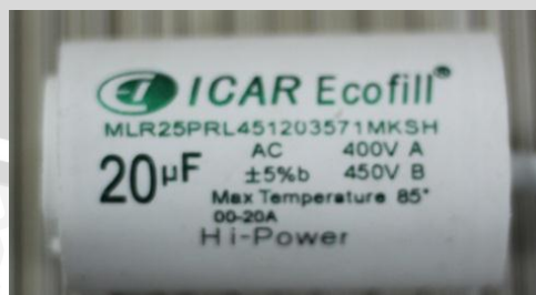
Gambar 4. 11 Kapasitor AC merek ICAR Ecofill 20 \mu\text{F}
