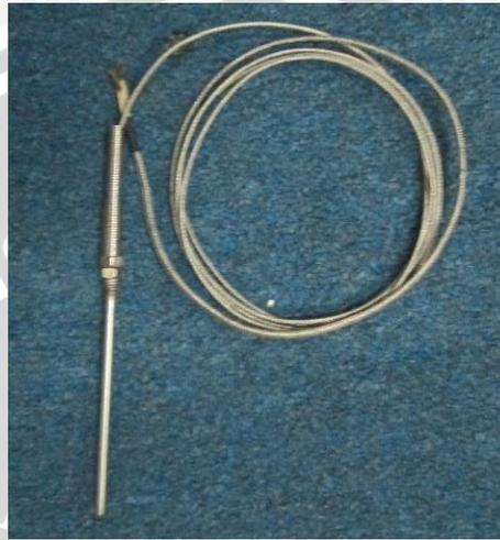
Gambar 3.5 *Thermocouple* tipe k
