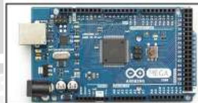
Gambar 4. Arduino Mega
