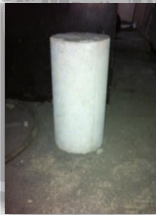
(a) Silinder Beton
