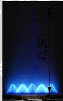
Gambar 4.8 Nyala Api *Perforated Burner* Rasio Ekuivalen 1.2
