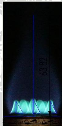
Gambar 4.9 Nyala Api *Perforated Burner* Rasio Ekuivalen 1.45
