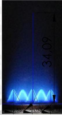
Gambar 4.7 Nyala Api *Perforated Burner* Rasio Ekuivalen 1.03
