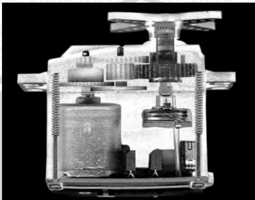
Gambar 2.11 Bagian internal motor DC servo Sumber: Sawicz (2002:9)
