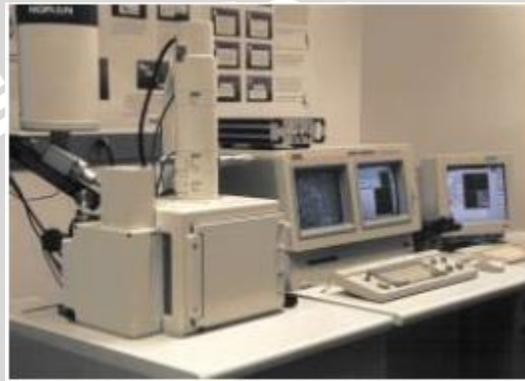
Gambar 2.8 Alat Scanning Electron Microscopy (SEM)
