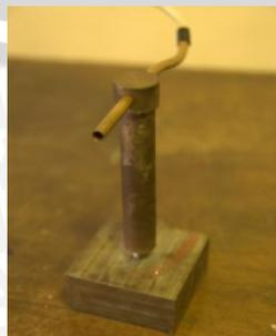
Gambar 3.10 *Combustor holder*
