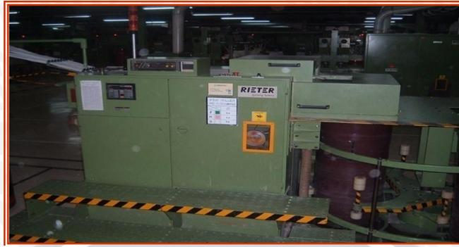
Gambar 4.5 Mesin *Pre Drawing*
