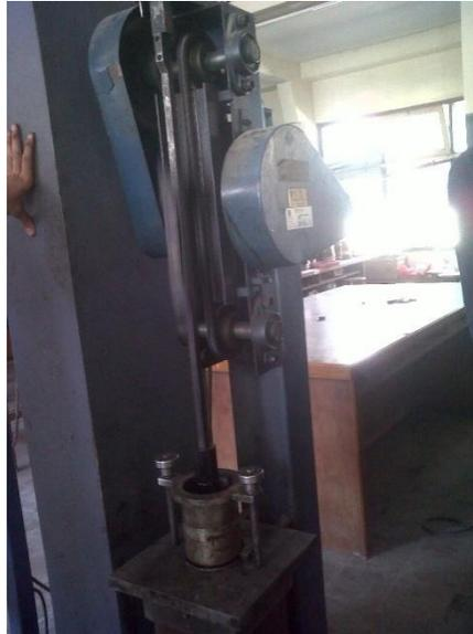
*Gambar 3.2 Foto Automatic Asphalt Compactor*
