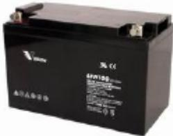
The rechargeable batteries are lead-lead dioxide systems. The dilute sulfuric acid electrolyte is absorbed by separators and plates and thus immobilized. Should the battery be accidentally overcharged producing hydrogen and oxygen, special oneway valves allow the gases to escape thus avoiding excessive pressure build-up. Otherwise, the battery is completely sealed and is, therefore, maintenance-free, leak proof and usable in any position.
