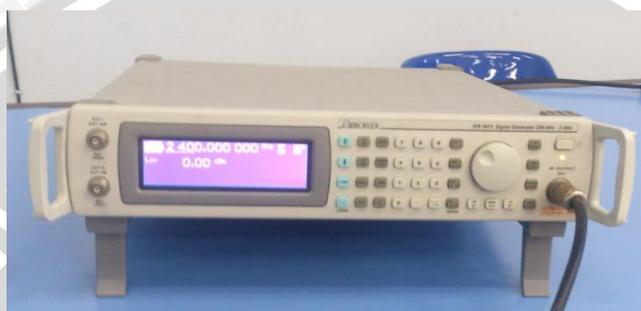
**Gambar 64.** Aeroflex IFR 3413 *Signal Generator* 250 KHz - 3 GHz
