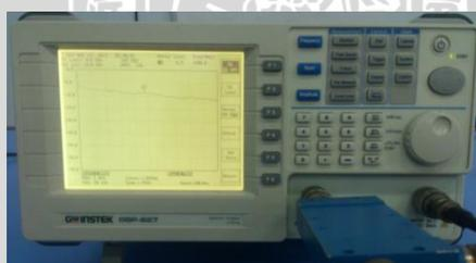
**Gambar 61.** GW Instek Spectrum Analyzer 2,7 GHz
