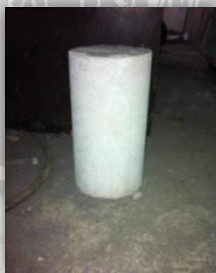
(a) Silinder Beton
