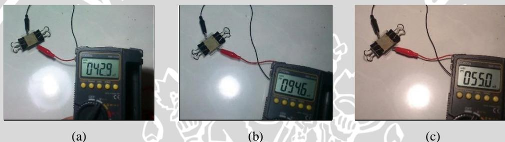
Gambar 5.11 Hasil Uji Voc DSSC 2 Menggunakan Lampu CFL (a), LED *Cool Daylight* (b), LED *Warm White* (c)
