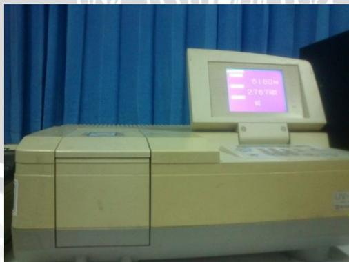
Gambar 5.1. *UV-VIS Spectrophotometer (Shimadzu)* tipe *UV – 1601*
