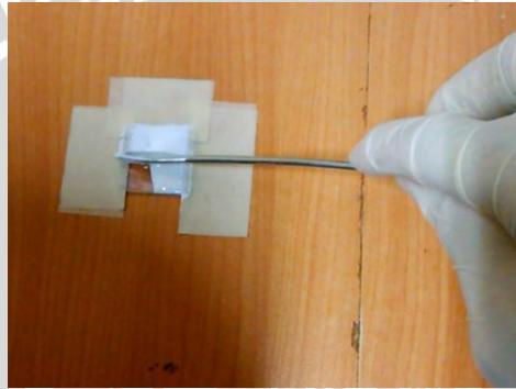
Gambar 4.8 Proses Pelapisan Pasta  $\text{TiO}_2$
