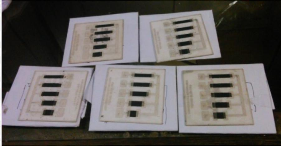
Gambar 4.16 Resistor hasil proses film tebal
