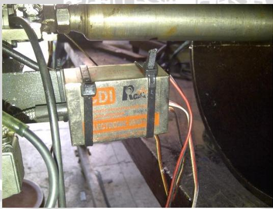
Gambar 4.6 *Capacitor Discharge Ignition (CDI)*
