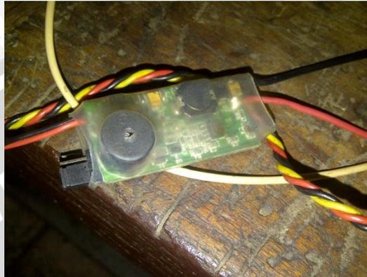
Gambar 4.7 UBEC (*Universal Battery Elimination Circuit*)
