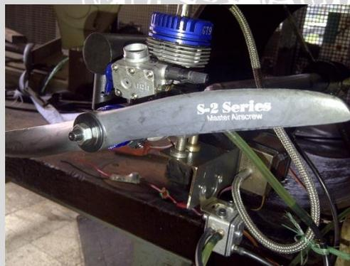
Gambar 4.8 Propeller tipe *S2 series* 11 x 5 inch.
