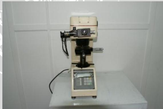
Gambar 3.4 *Microvickers hardness apparatus*
