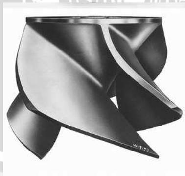
Gambar 2.12 Mixed flow *impeller*
