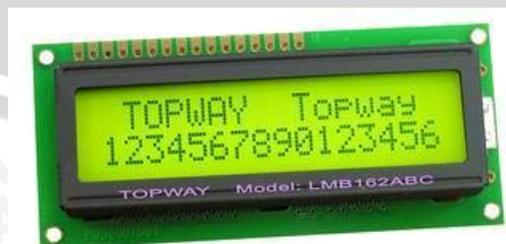
Gambar 2.11 LCD (*Liquid Crystal Display*) LM162A
