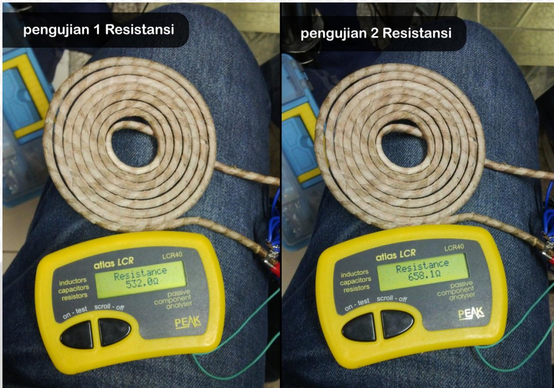
Gambar 5. 1. Pengujian nilai resistansi pancake coil
