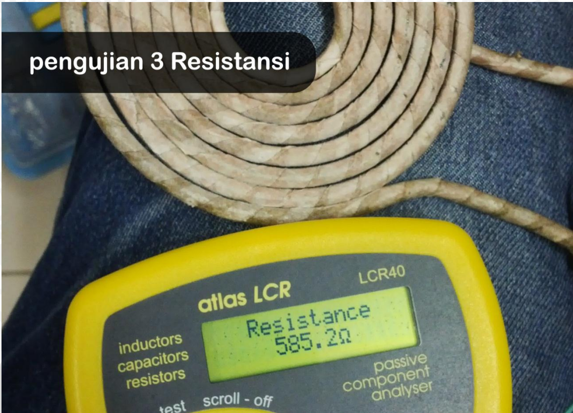
Gambar 5. 2 Pengujian nilai resistansi pancake coil
