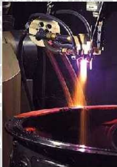
Gambar 2.4 Proses Thermal Spray Coating Sumber: Anonymous3.2013
