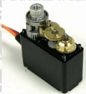
Gambar 2.18 Sistem Mekanik Motor Servo
