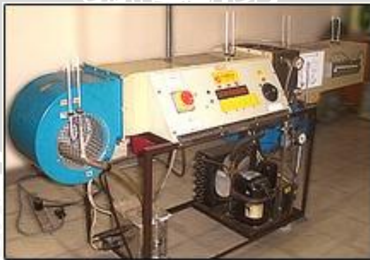
Gambar 3.1 Instalasi AC Bench PA Hilton
