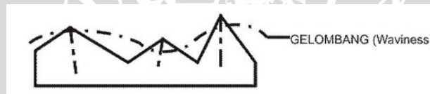
Gambar 2.11 Gelombang / waviness (macroroughness) . Sumber: Anonymous 1 (2012:225).
