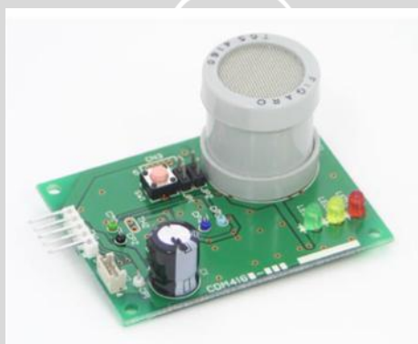
Gambar 2.5 Modul sensor CO 2 CDM4160 Sumber: Datasheet CDM4160
