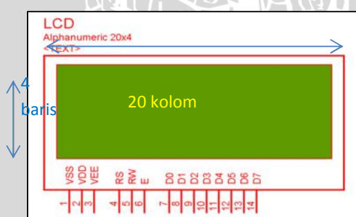
Gambar 2.13 Konfigurasi Pin LCD Karakter 4X20 Sumber: Software Proteus ISIS Schematic Library, 2009
