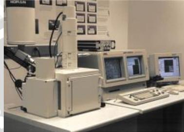
Gambar 2.6 *Scanning Electron Microscope*
