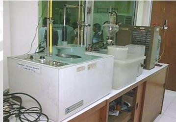
Gambar 3.5 Bomkalorimeter
