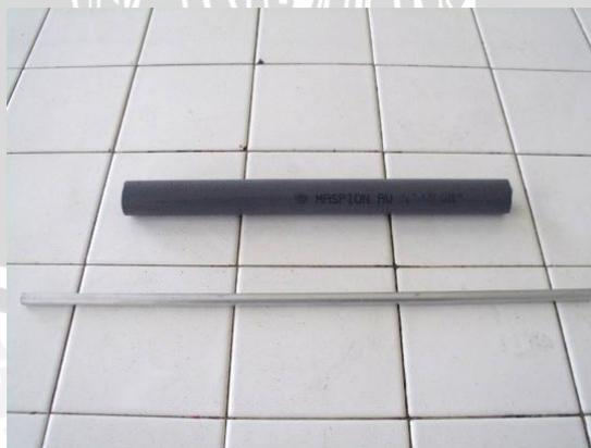
Gambar 3.5 Pipa PVC dan aluminium
