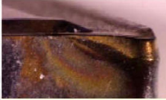
**Gambar 2.10.** Deformasi Plastis (*Plastic Deformation*)
