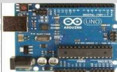
Gambar 2.37 Board Arduino Uno berbasis ATmega 328P
