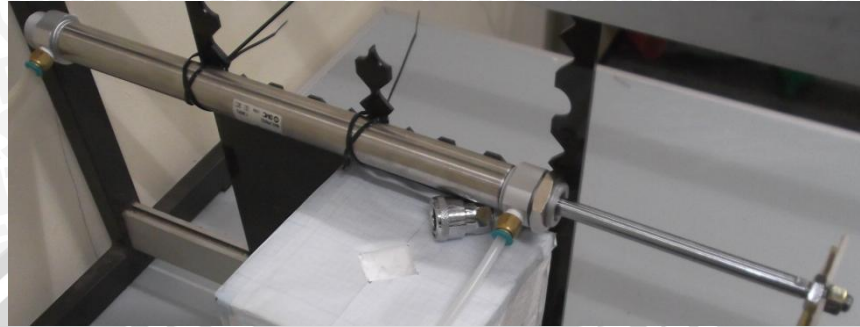
Gambar 4.7 Silinder Double Acting SMC CDM2b25-300
