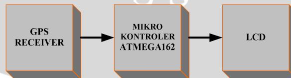
Gambar 5.1. Diagram Blok Pengujian GPS *Receiver*
