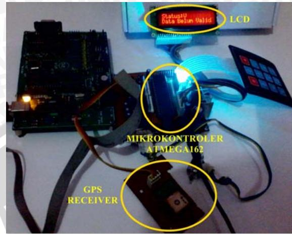
Gambar 5.2. Pengujian GPS *Receiver* (Data Belum Valid)
