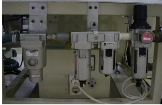
Gambar 2.6 Separator Mesin Sucking Blowing Sumber : Sucking Blowing Machine PT OMI.
