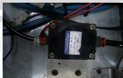
Gambar 2.8 Air valve Sucking Blowing Machine. Sumber : Sucking Blowing Machine PT OMI.
