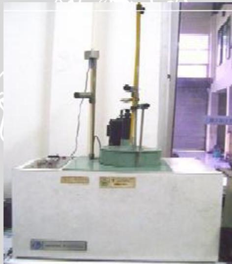
Gambar 3.8 Bomb Kalorimeter
