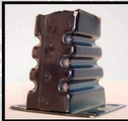
Gambar 2.6 Crash box tabung berpenampang bergelombang (*corrugated tubes*)
