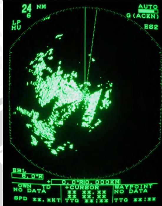
Gambar 5.43. Tampilan *Display Radar Furuno Dengan A/C Rain 1 Skala*
