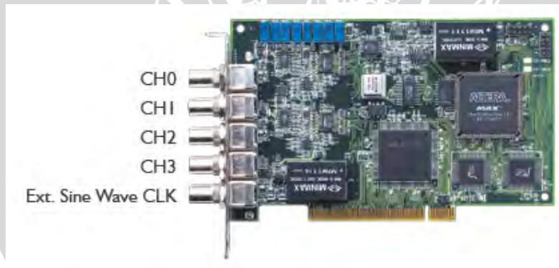
Gambar 2.17. ADC ADLINK PCI-9810.
