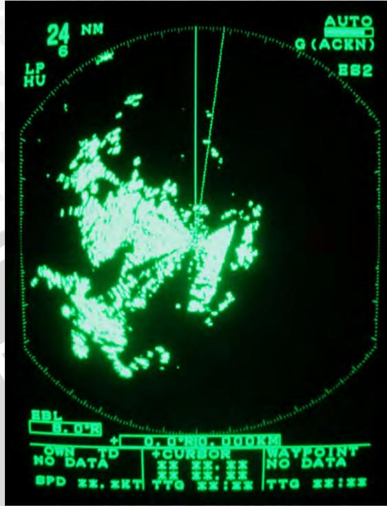
Gambar 5.41. Tampilan *Display Radar Furuno* Dengan A/C *Rain 1/2* Skala
