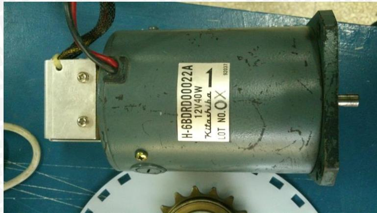
Gambar 1.3 Motor DC Magnet Permanen 12 V
