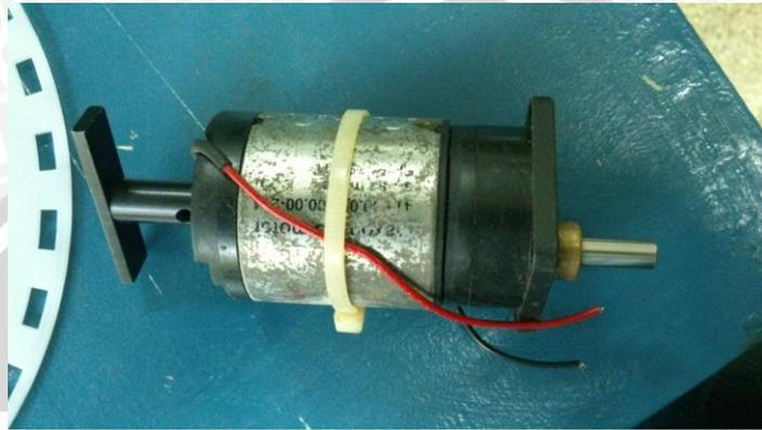
Gambar 1.4 Motor Simulator Roda Sepeda
