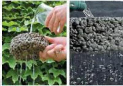
**Gambar 2.6** *Porous concrete*
