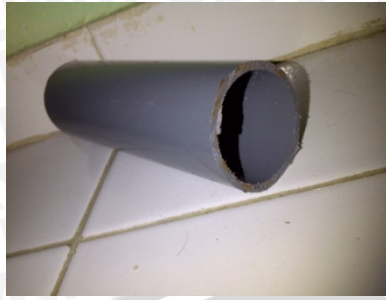
Gambar 3.3 Pipa PVC 1,25 inch.
