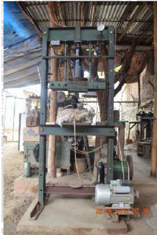
Gambar 3.5 Instalasi Penelitian (a) Instalasi mesin hot pressing , (b) Mesin hot pressing .
